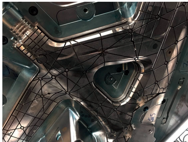
Fig. 2. Shrinkage and warpage during injection molding were calculated by simulation and the position and wall thickness of reinforcing struts inside the frame were improved
